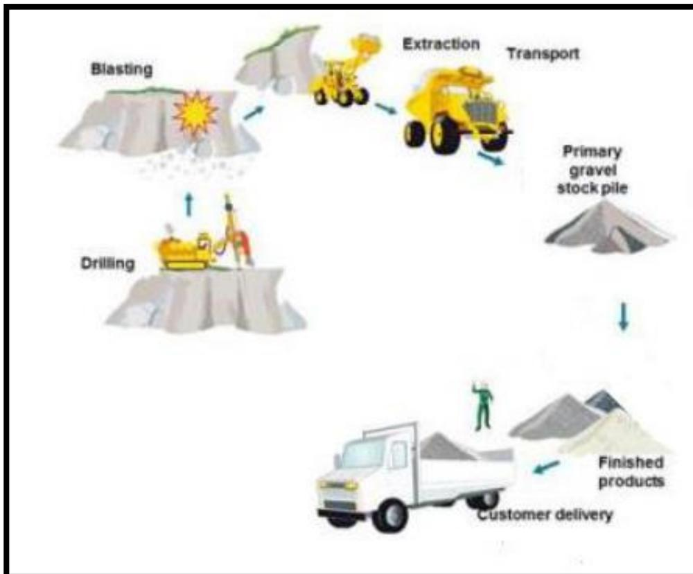
Figure 2: Operation Plan of the proposed Quarry.
