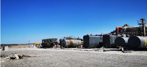
**HAZARDOUS AREA – BUNDING WALL TO BE INSTALLED SURROUNDING ENTIRE LAYED WITH CONCRETE FLOOR**
