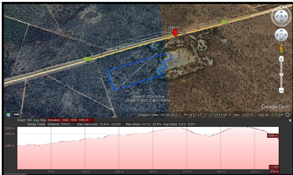
Figure 2: Elevation profile of the proposed mining footprint (Image obtained from Google Earth)
