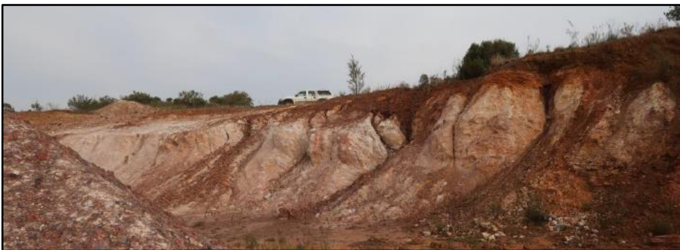
Figure 45: Profile showing cleaner kaolinite close to the surface in the east of the area, looking south (Images obtained from the PIA).
