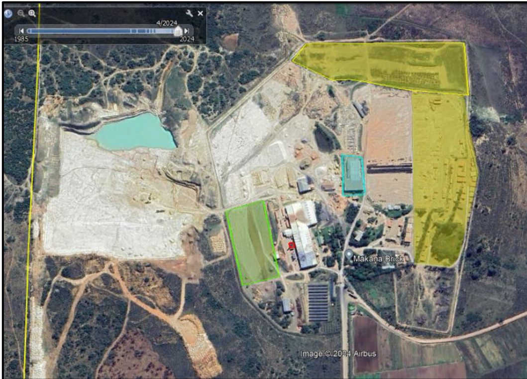
Figure 1: Satellite view of the stockpile area that was reinstated (green polygon), Plant 1 that will no longer be used (blue polygon), and the areas earmarked for rehabilitation (yellow polygons).
