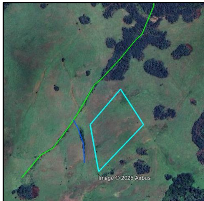
Figure 24: Satellite image of the earmarked area (light blue polygon) in relation to the drainage line (dark blue line), and the small stream (green line) (image obtained from Google Earth).
