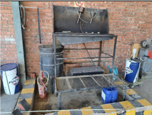
Bund at workshop
