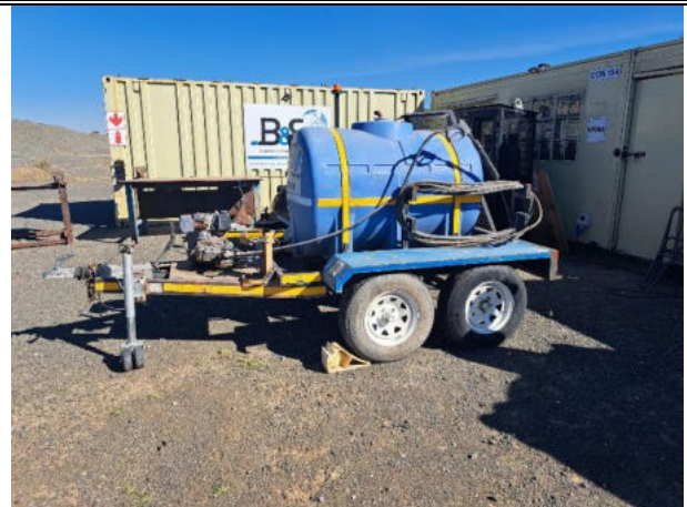
Drip trays and/or bunds to be added. Alternatively the equipment must be removed from site
