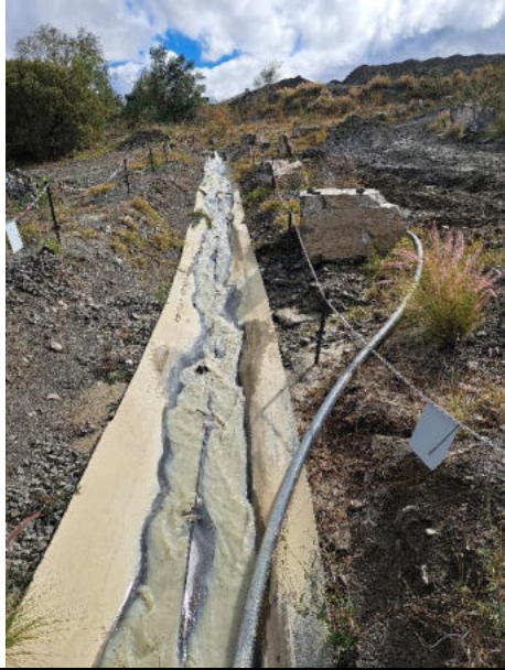
Conveyor belts used to direct the water runoff from the sand plant to the settling ponds
