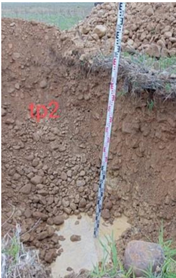
Figure 4. Typical soil profiles in test pits on the site.
