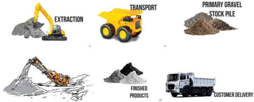
Figure 2: Operation Plan of the proposed site.
