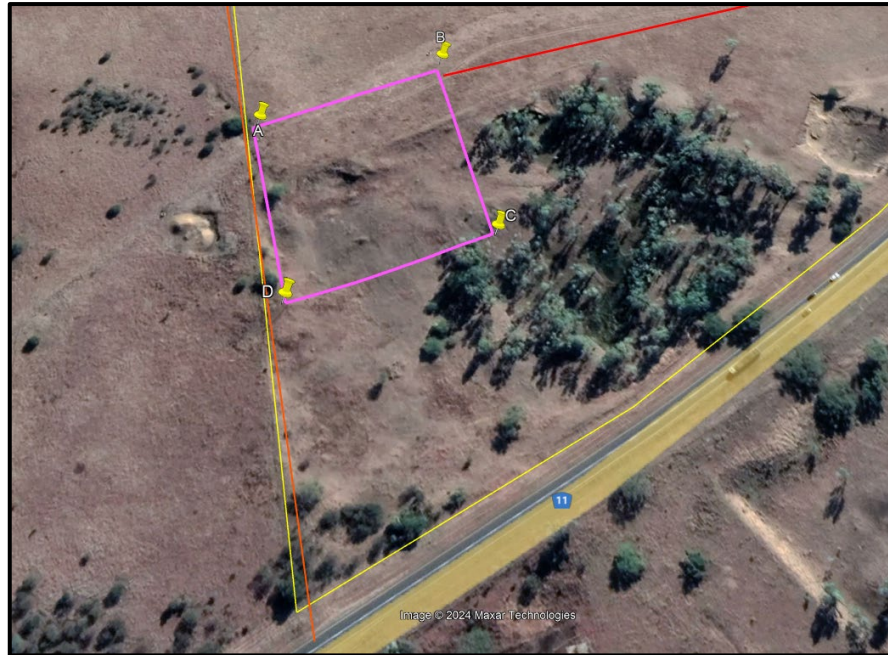
Figure 4: All mining will be >10 m from the adjacent power lines (orange line) (image obtained from Google Earth).
