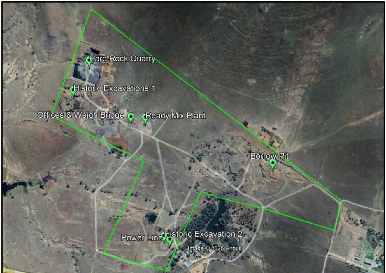
Figure 1: Satellite view of the layout of the Thaba Stone Quarry (image obtained from Google Earth).
